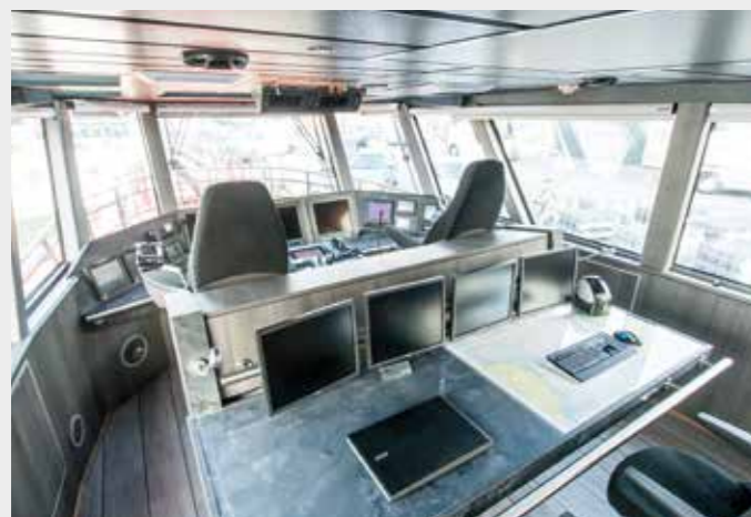
The bridge has two helmsman's seats and a survey console with a further two seats
