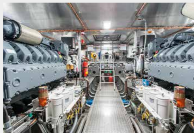
The propeller shafts are driven by two MAN V12 main engines
