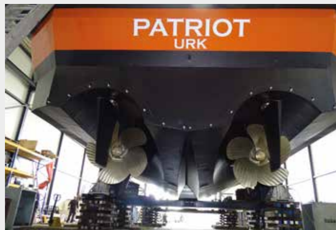
The hull has tunnels in way of the twin propellers
