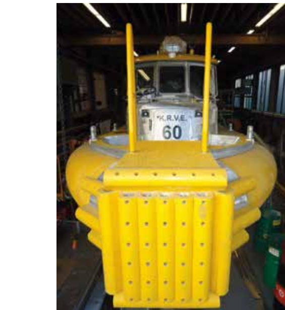
New fendersystem for the fast crew tender KRVE 60 vessel by Poly Marine Fender Systems.
